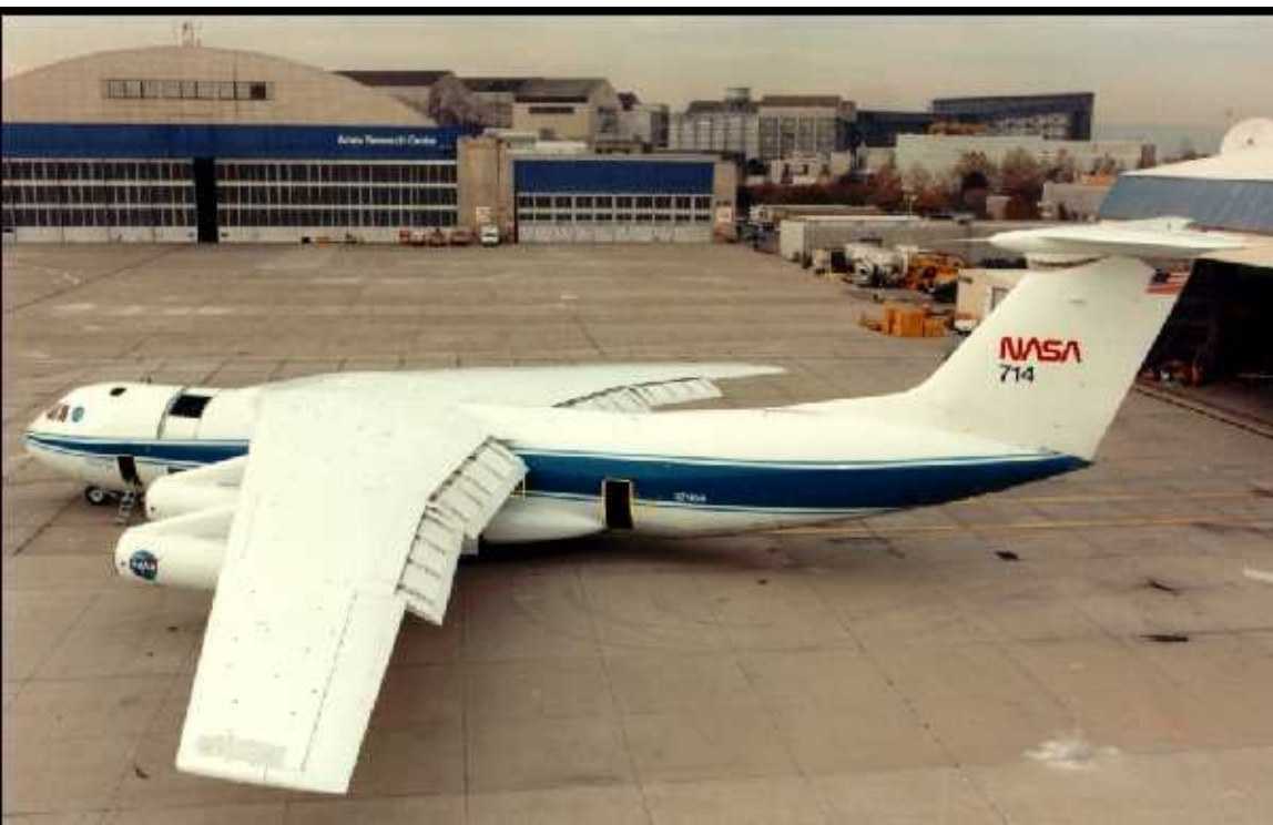
NASA's Kuiper Airborne Observatory (KAO) C-141 with a 36-inch telescope onboard, based at NASA-Ames near San Francisco, flew from 1975 - 1996
